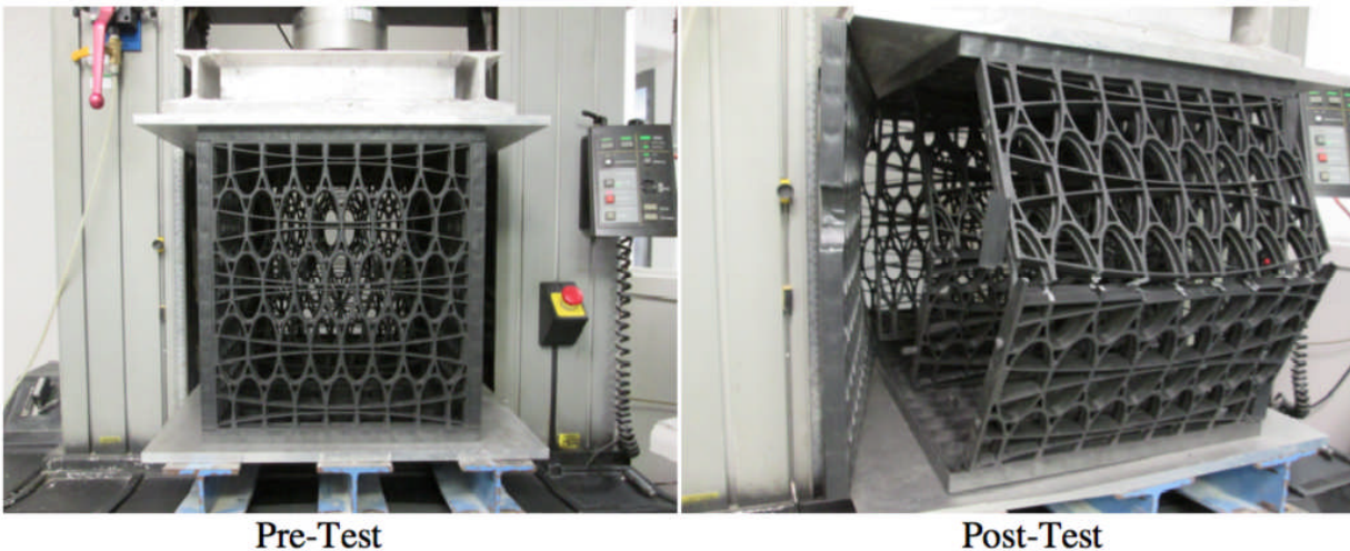
Figure 2: Parallel plate loading of R-Tank module
